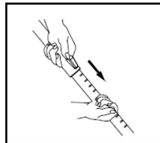
2. Adjust the length of the telescopic tube by pushing the locking mechanism down and pulling out the bottom section of the tube to a suitable length.
