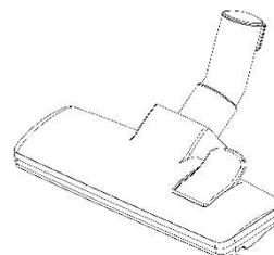
**Please note** this tool can be used either with the extension tube or directly onto the vacuum cleaner for closer cleaning.
