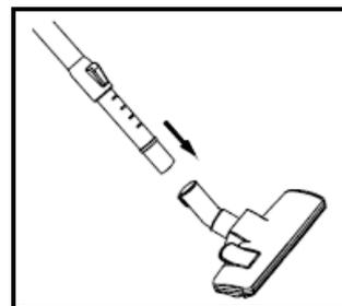
3. Fit the floor nozzle into the telescopic tube.
